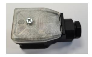
Connect the yellow/green wire to the connector insert using the PE terminal. Make sure that the 2 notch highlighted below is facing right. Do not conect the neutral and phase wires.
