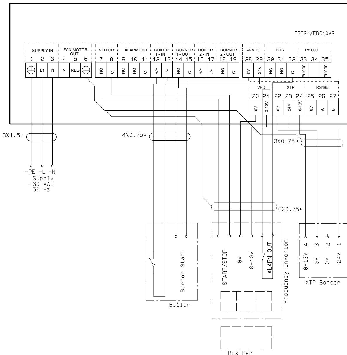
This example shows how to connect a PDS to EBC10v2. The PDS supplies extra monitoring
