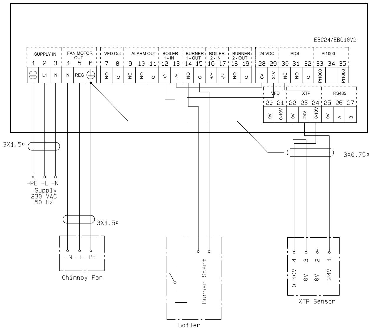
The example shows how a voltage signal (24 V DC) is connected to EBC10v2 for the chimney fan to run continuously.
