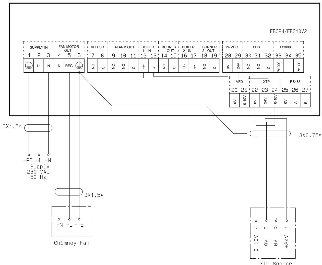
This example shows how to connect a voltage signal (23 V DC) to EBC10v2 to start the chimney fan.
