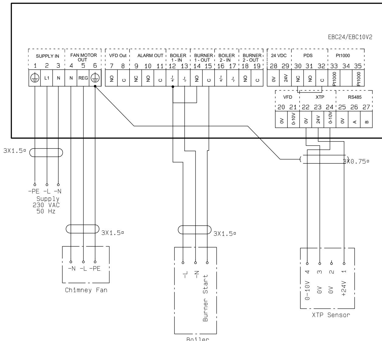
This example shows how to connect a voltage signal (18-230 V AC/DC) to EBC10v2 to start/stop the chimney fan.
