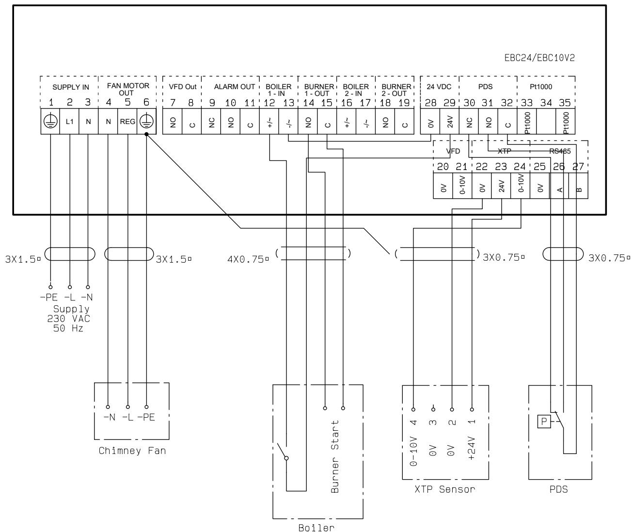
This example shows how to connect a potential free contact to the EBC10v2 to start/stop the fan:
