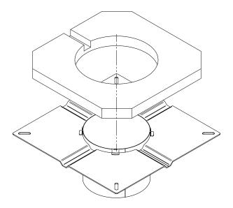
Fixate the flange to the cover plate with the use of the vibration dampers supplied with the flange.
