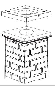
Now the chimney fan with the location brackets can be install on the brick chimney.
