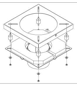
4 Fixate the flange and cover plate assembly to the chimney fan.
