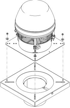
Now the chimney fan with the cover plate and flange can be install on the steel chimney.
