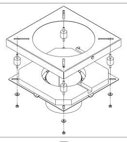
Fixate the flange and cover plate assembly to the chimney fan.
