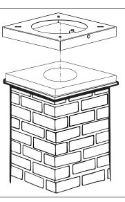
Now the chimney fan with the location brackets can be install on the brick chimney.
