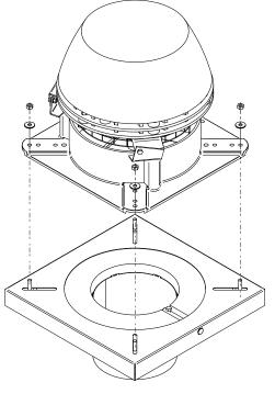
Now the chimney fan with the cover plate and flange can be install on the steel chimney.
