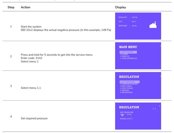
**Note!** This procedure only covers setting the pressure in the chimney.
