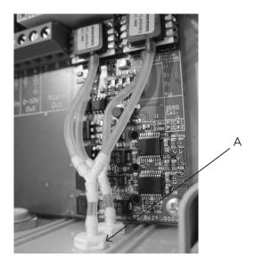
For outdoor installation, place the pressure transducer where it is not exposed to the weather. For outdoor installation, the pressure transducer should be placed in a box fitted with a hole (Ø2mm) in the bottom. The hole serves to ensure correct reference pressure and prevent water entry
