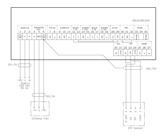
The example shows how a voltage signal (24 V DC) is connected to EBC24 for the chimney fan to run continuously
