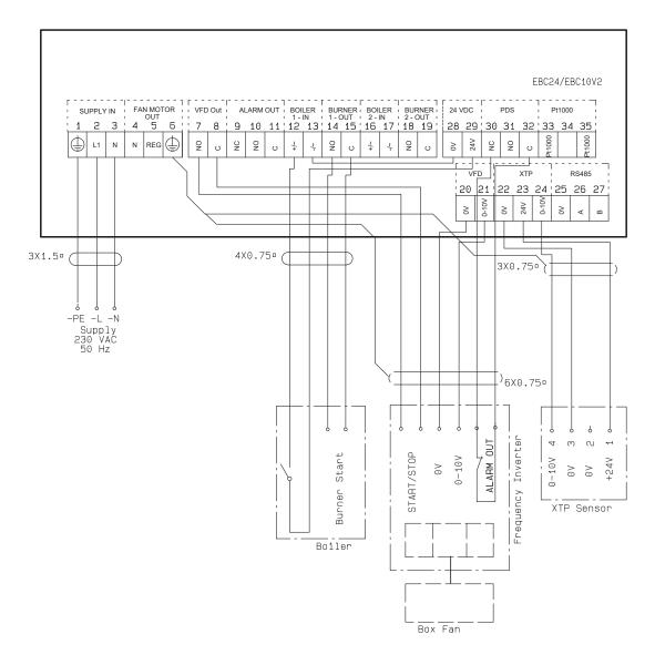
This example shows which inputs/outputs on the EBC24 need to be connected to the frequency inverter/ MPR-relay:
