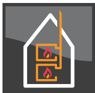
Decentralized multiple fireplaces connected to same chimney
