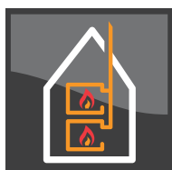
Decentralized multiple fireplaces connected to same chimney
